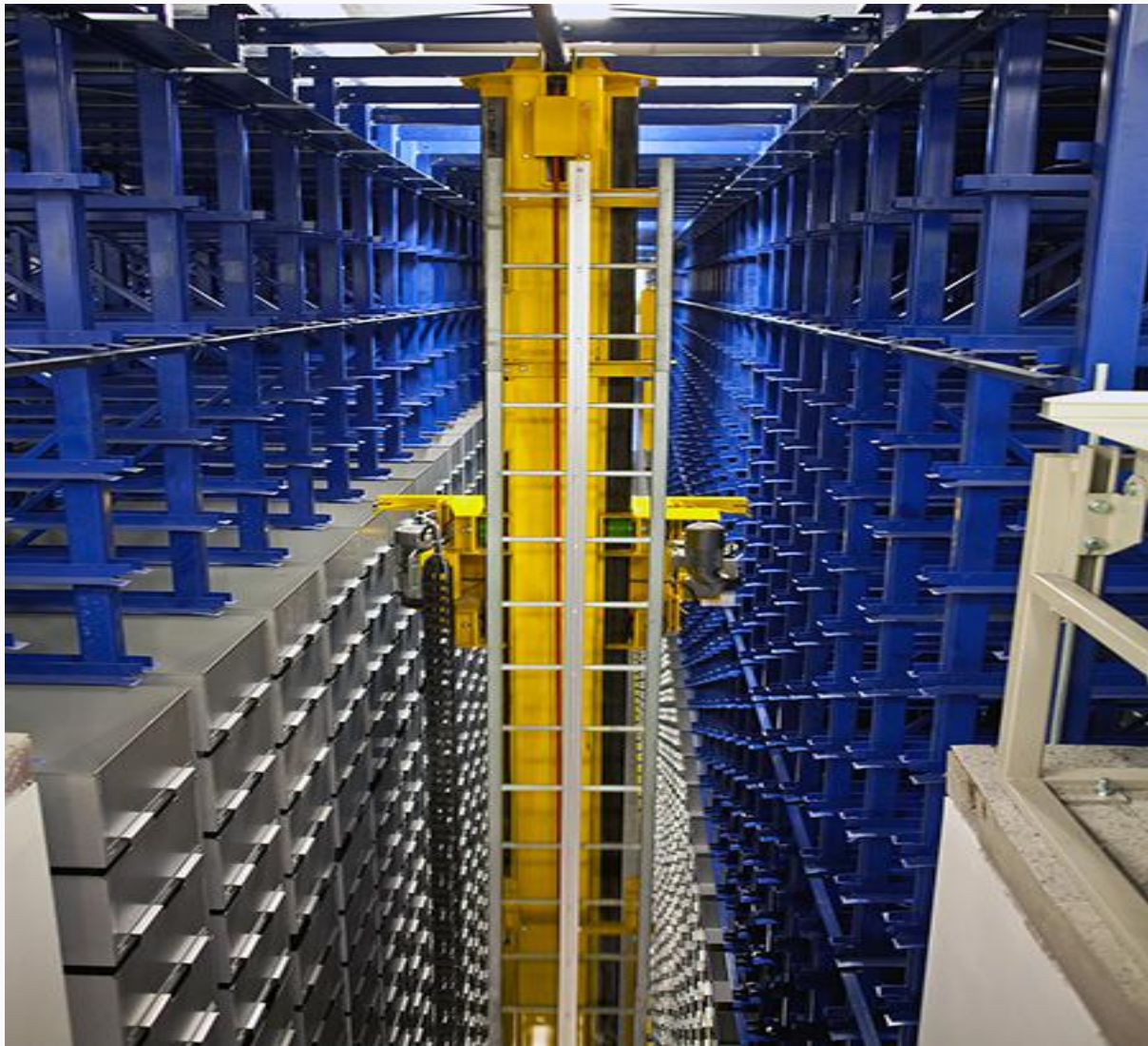
Books and other materials are stored in bins that are retrieved robots
